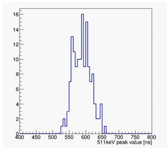
The PET exhibits an average of about 12% energy resolution. As  $V_{op}$  is increased, each MPPC channel reaches saturation, which degrades energy resolution. As such, over voltage must be set to the optimum value (not too high) by taking into account energy resolution characteristics.
