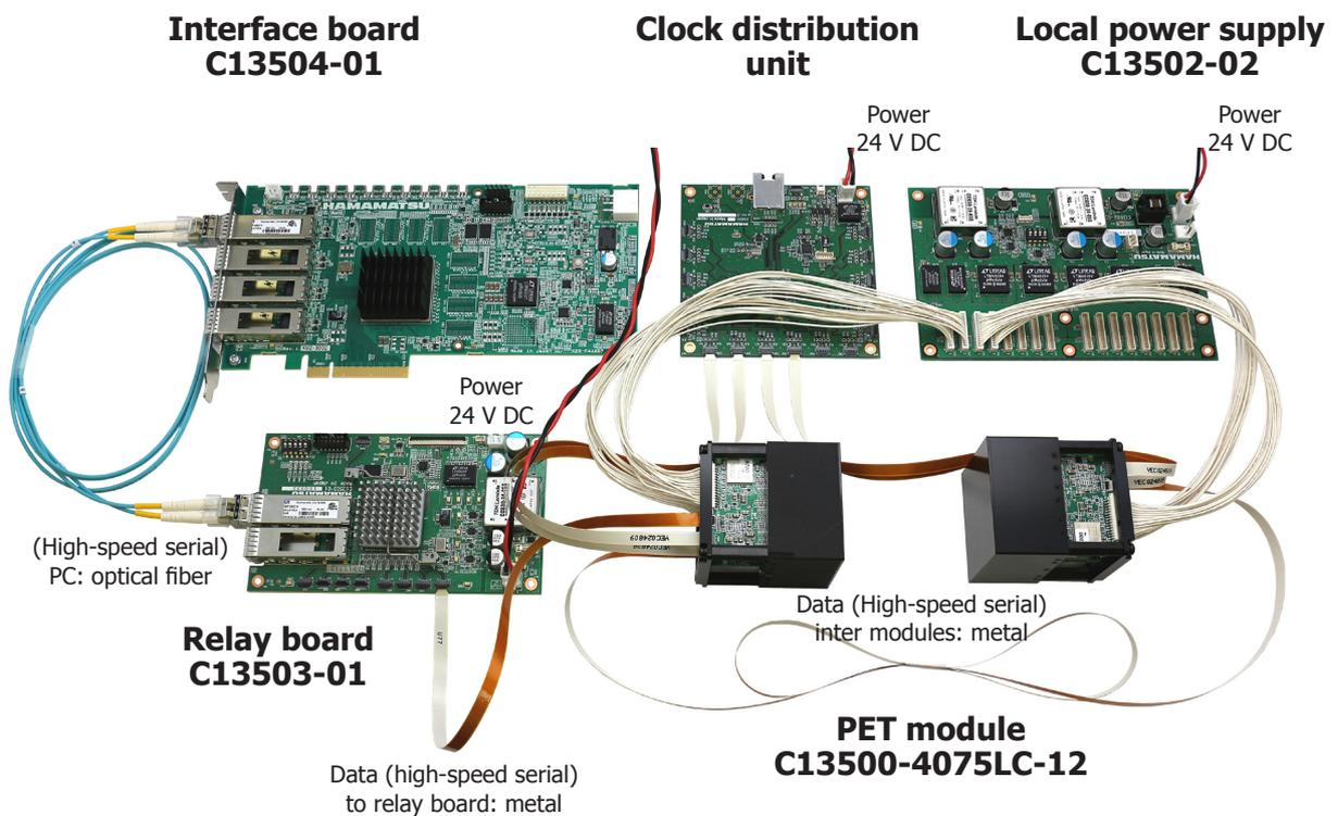
The signal processing boards of each PET module are connected in a cascaded fashion, and the last board is connected to the relay board C13503-01. The relay board is connected to the interface board with a fiber optic (SFP).
