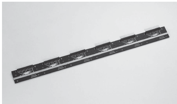
[Figure 6-5] Long and narrow image sensor consisting of multiple photodiode arrays with amplifiers
