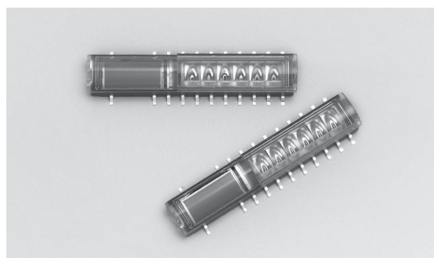
[Figure 3-6] Light emitting/receiving module P8212 for VICS
