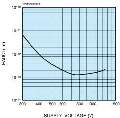
Data shown here, which is given from a relation among supply voltage, anode sensitivity and dark current, serves as a good reference in order to determine the most suitable supply voltage or its range.
