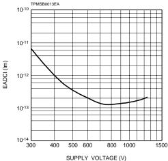
Data shown here, which is given from a relation among supply voltage, anode sensitivity and dark current, serves as a good reference in order to determine the most suitable supply voltage or its range.
