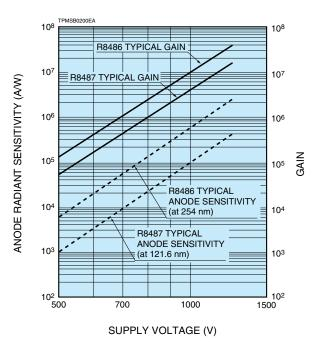
Figure 2: Typical Gain and Anode Radiant Sensitivity
