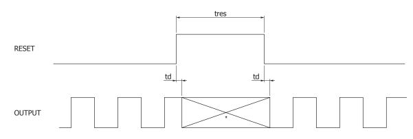
\* OUTPUT terminal is at High impedance during RESET period ("High" state).
