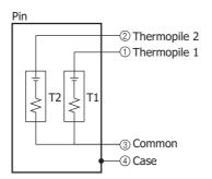
Filter1: For reference (3.9  $\mu$ m) Filter2: For CO<sub>2</sub> (4.3  $\mu$ m)
