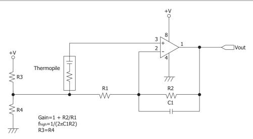
Since the thermopile output signal is very low in the order of microvolts, use an amplifier with a low offset voltage. (Example: LTC1050)
