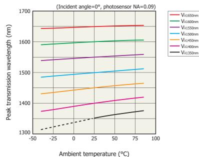
The broken line corresponds to data when the built-in band-pass filter is removed. The C14272 cannot detect the peak transmission wavelength accurately in this range. This is because when the ambient temperature is less than 25 °C, the peak transmission wavelength of the MEMS-FPI tunable filter is outside the transmission wavelength range of the band-pass filter.
