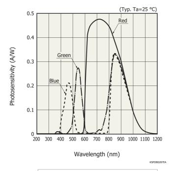
Since this photodiode has sensitivity in the infrared region, infrared light must be filtered out as needed.
