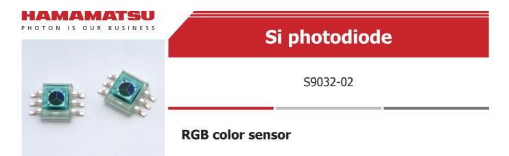
The S9032-02 is a color sensor molded into a plastic package having a 3-channel (RGB) photodiode sensitive to the blue ( $\lambda p$ =460 nm), green ( $\lambda p$ =540 nm) and red ( $\lambda p$ =620 nm) regions of the spectrum. The S9032-02 has a 3-segment (RGB) circular photosensitive area of  $\phi 2$  mm.
