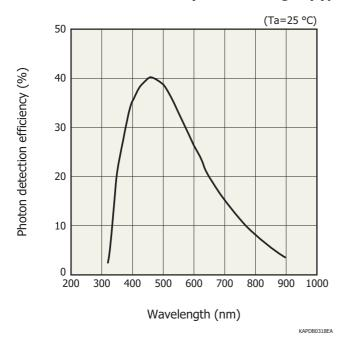
Photon detection efficiency does not include crosstalk or afterpulses.
