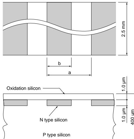
S8380 series: a=50  $\mu\text{m}$ , b=45  $\mu\text{m}$
