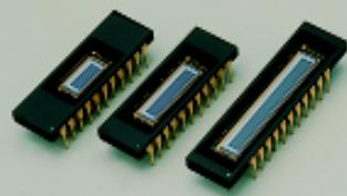
S8380/S8381 series are designed to have higher sensitivity in the infrared and soft X-ray regions when compared to standard NMOS linear image sensors. The peak sensitivity wavelength is in the near IR region ( $\lambda_p=750$  nm).
