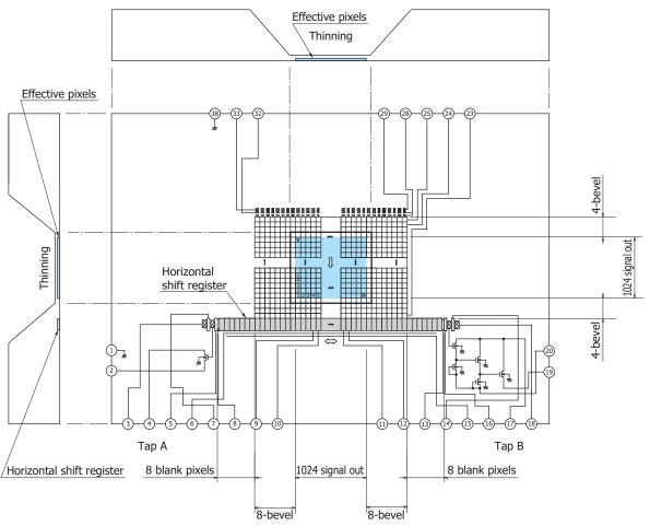
Note: When viewed from the direction of the incident light, the horizontal shift register is covered with a thick silicon layer (dead layer). However, long-wavelength light passes through the silicon dead layer and may possibly be detected by the horizontal shift register. To prevent this, provide light shield on that area as needed.
