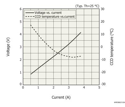
To make the cooling side 0 °C, the temperature on the heat dissipating side must be 30 °C or less. As a guideline, use a heatsink whose thermal resistance is no more than 1 °C/W.
