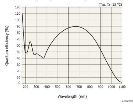
\*16: Spectral response is decreased according to the spectral transmittance characteristics of window material.
