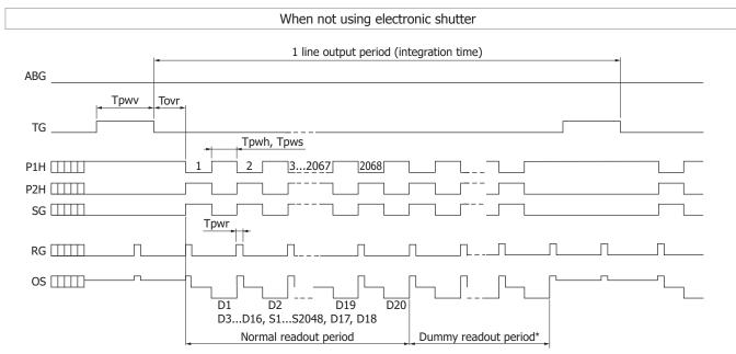
\* When making the integration time longer than the normal readout period, to carry away the dark current generated in the CCD horizontal shift register, perform dummy readout after completion of the normal readout until right before rising transfer gate pulse.
