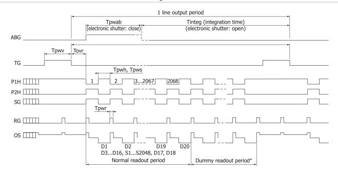
\* When making the integration time longer than the normal readout period, to carry away the dark current generated in the CCD horizontal shift register, perform dummy readout after completion of the normal readout until right before rising transfer gate pulse.
