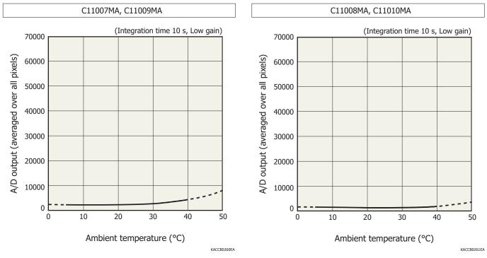
A/D output is the sum of the sensor and circuit offset outputs and the sensor dark output.
