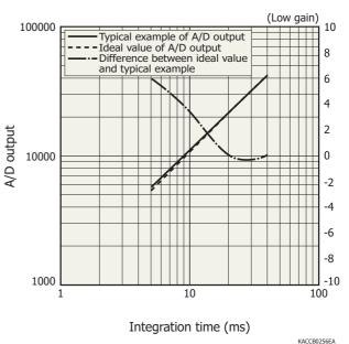
A/D output is the output with dark output is subtracted when light is input. The difference between the ideal value and typical example contains a measurement error. The smaller the A/D output, the larger the measurement error.
