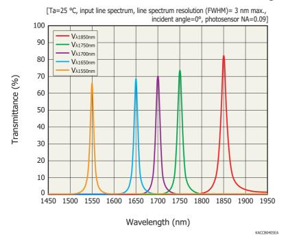
There is tolerance in filter control voltage for arbitrary peak transmission wavelength from unit to unit. The individual data for  $V\lambda1850nm$  and  $V\lambda1550nm$  at Ta=25 °C is to be described in an inspection sheet attached with a product on delivery.
