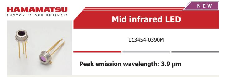
The L13454-0390M is a high-output mid-infrared LED with a 3.9  $\mu$ m peak emission wavelength. It is a product that has been achieved using Hamamatsu unique crystal growth technology and process technology. It is a suitable reference light source for gas measurement.
