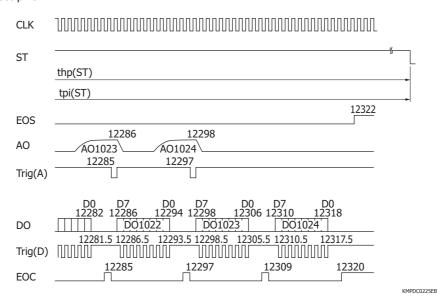
Note: When using analog output AO, read the AO output at the falling edge of Trig(A). When using digital output DO, read the DO output at the falling edge of Trig(D).
