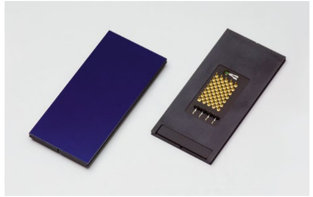
CCD image sensors installed in the Hyper-Suprime Cam
